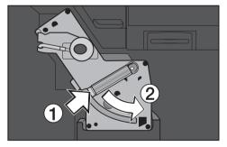
■ Press the light colored button on the brew unit handle, ①, and turn the handle to the right, ②.
